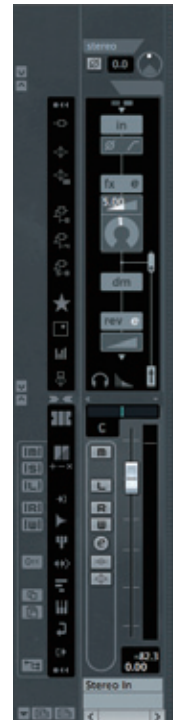
▶ screen 4 : When used with Steinberg Cubase, the dedicated input setting screen will be displayed within Cubase where you can set gain, +48V phantom power supply, phase inversion, and REV-X's send amount without opening dspMixFx. Depending on the insert point of SWEET SPOT MORPHING CHANNEL STRIP, you can record with effects as well as monitor.
