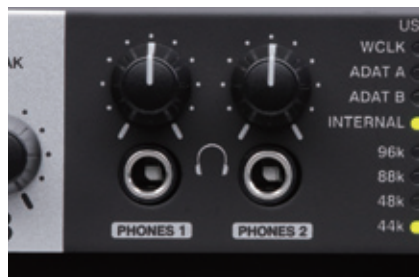
▲Picture 4 : Just like UR28M, there are 2 headphone outs. Each out can be monitored by any mix balance from Mix 1 to 4 which is set by dspMixFx.
