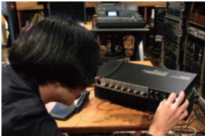
▲Picture 1 : This is me, checking UR824. By adding ADAT input/output, 24 in/24 out can be used and only 1 USB cable is needed to do this. This unit can be the center device of the studio.
