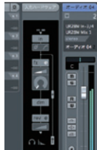
▲Picture 2: 4-step level meters are available for both input and output. The red indicates level over, the 2 oranges under the red indicate higher than -3 dB/-14 dB respectively and the green indicates higher than -48 dB.
