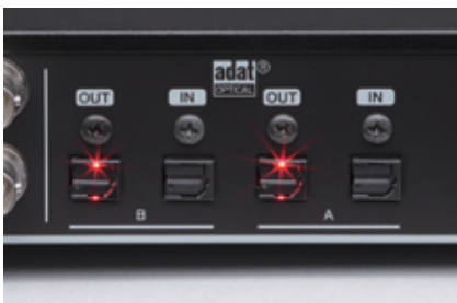
▲Picture 3 : ADAT optical jack on the rear. It supports S/MUX. When working at normal 48kHz, you can use 2 outs for 16 in/16 out, even at 96kHz, you can use 8 in/8 out.
