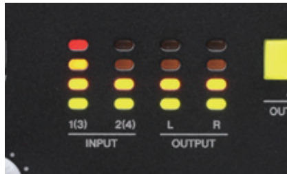
▲Picture 2: 4-step level meters are available for both input and output. The red indicates level over, the 2 oranges under the red indicate higher than -3 dB/-14 dB respectively and the green indicates higher than -48 dB.
