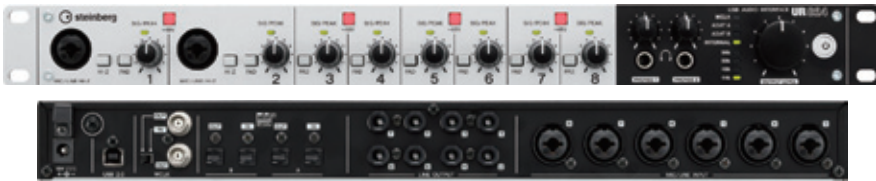
▲UR824's front and rear. In the front, there are Mic/Line inputs for 2 channels (XLR/TRS phone combo), gain knobs for all the analog inputs and 2 headphones (stereo phone). On the rear, from left, USB2.0, word clock input/output (BNC), 2 ADAT optical input/output (can be switched to S/P DIF), 8 Line output (TRS phone) and 6 Mic/Line input (XLR/TRS phone combo).
