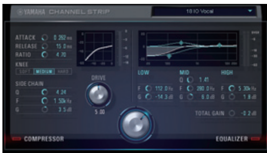
▲ screen 2 : A dspMixFx's DSP effect, SWEET SPOT MORPHING CHANNEL STRIP. The Morph knob in the center has 5 comp/EQ settings recorded for each preset. As you turn the knob, the parameter value changes just like it is morphing.
