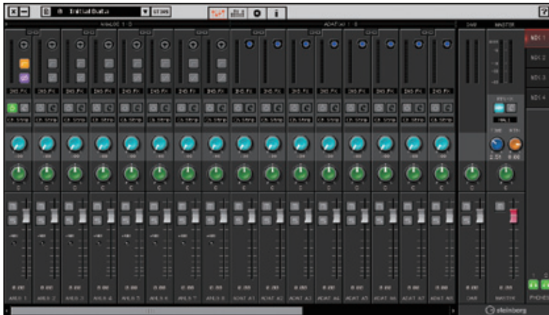
◀ screen 1 : Dedicated DSP mixer software, dspMixFx. As the screen shows, there are input channels including both analog and digital; output channels from DAW and master channel to output monitor mix. You can adjust the balance between each channel and create your own monitor mix. You can save up to 4 "MIXS".
