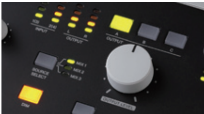
▲Picture 3: in the Alternate mode, the MIX selected in the SOURCE SELECT (refer to CLOSE-UP) will be output A to C. In the independent mode, each MIX will be output from each OUTPUT.
