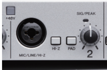
▲Picture 2 : Mic/Line input on the front. There is also HI-Z switch to directly switch on for high-impedance guitar or base. There is also -26dB PAD button
