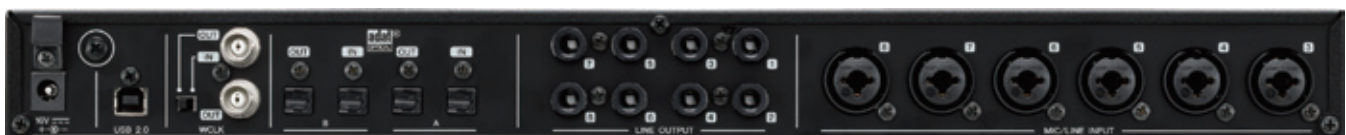
▲ On the rear panel, there are, from left, USB 2.0, word clock input/output (BNC), 2 ADAT optical inputs/outputs (switchable to S/P DIF), 8 Line outputs (TRS phone) and 6 Mic/Line inputs (XLR/TRS phone combo). On the front, there are 2 channels of mic/line/Hi-Z inputs (XLR/TRS phone combo).
